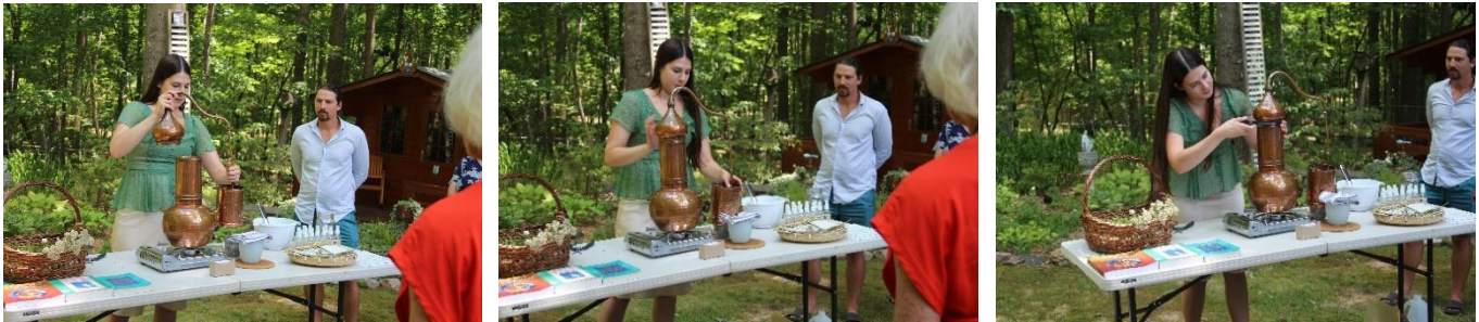
Left: Finishing the still assembly. Middle: Positioning the hydrosol collection pot. Right: Taping the top securely – the final step. The water is heated on a burner using a propane cylinder.
