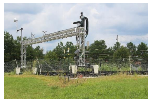
The weed ID teaching robot moves to the right on tracks.
